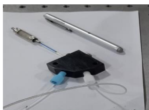
Sensing chamber with gas/vapour inlet and outlet.
