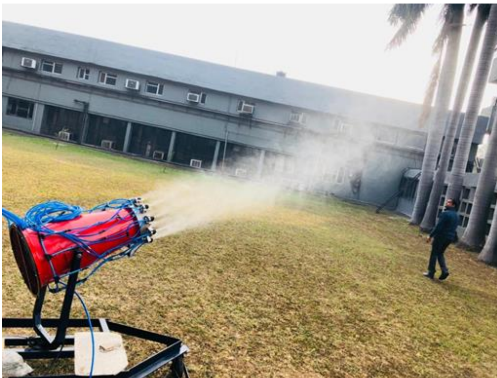
Experimental set-up of charging of liquid sprays for dust mitigation and smog control
