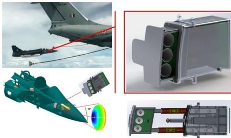
Drogue light functional system layout and fitment in LCA
