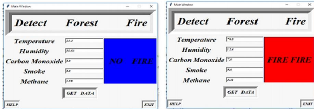
Sensor information in each node displayed in a GUI.
