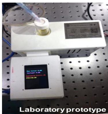
Sensing chamber with gas/vapour inlet and outlet.
