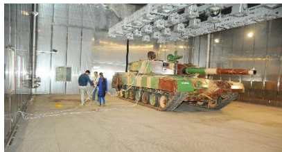
Prototype for measurement and analysis of temperature profile MBT-Arjun tank
