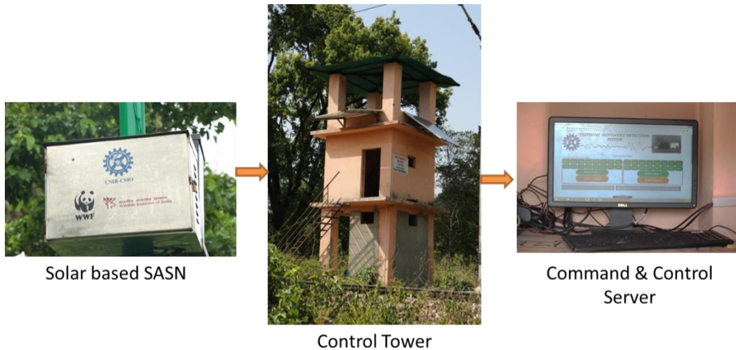
Layout of field nodes (SASN) with control server and user interface at Kansrao, RTR
