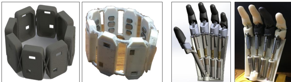
CAD model & fabricated prototype of EMG electrode band & of functional prosthetic hand
