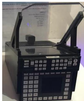
Lab prototype of HUD mk2 with digital interface and digital light engine as display source
