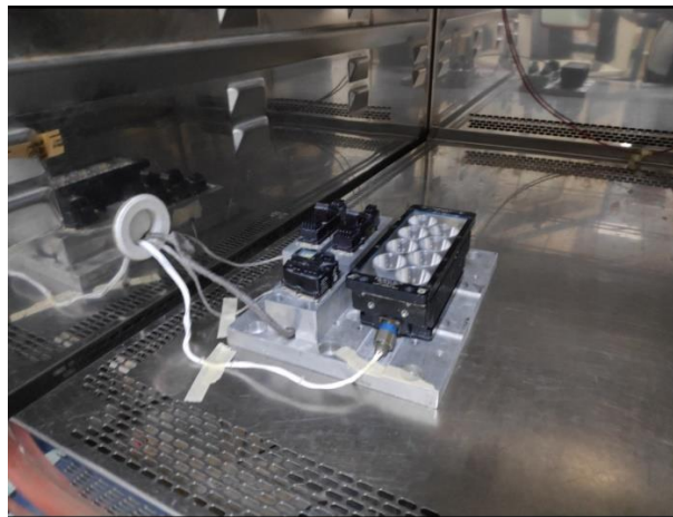
Taxi Landing Lights during Thermal Cycling (ESS Screening)
