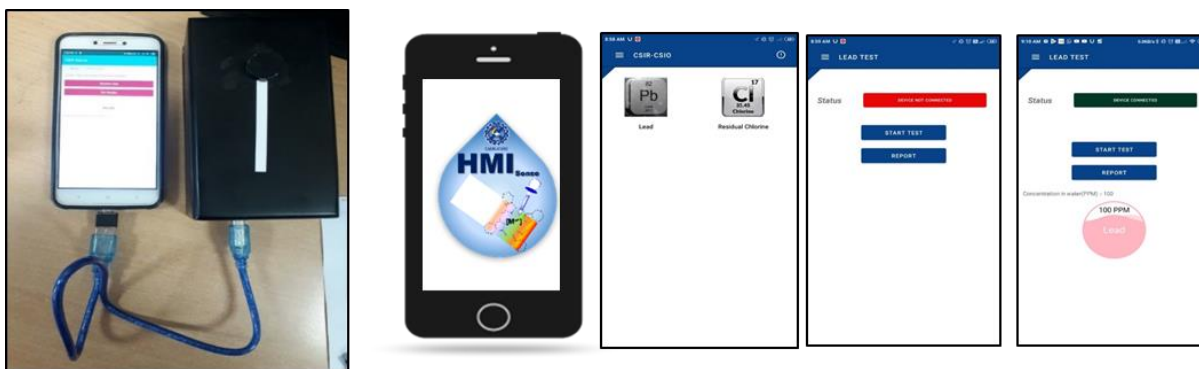
Mobile App, HMISense to Quantify Heavy Metals Level
