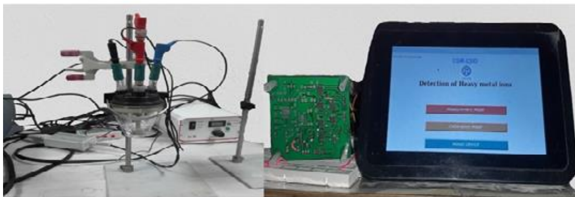
Lab-scale e-Tongue Prototype for Heavy Metal Detection in water
