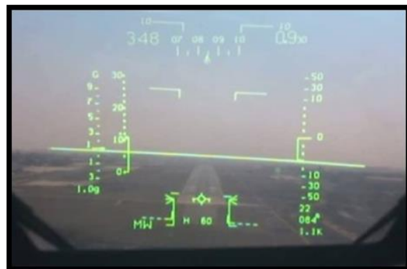
Flight Symbology viewed through HUD Mk1 in LCA-AF
