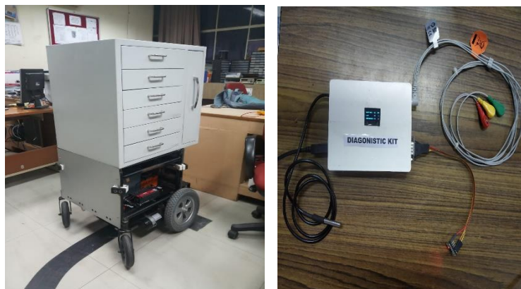
Robot trolley and diagnostic kit to monitor patient parameters
