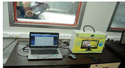
Prototype for measurement and analysis of temperature profile MBT-Arjun tank
