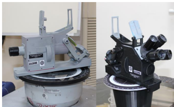
Functional Prototypes of Optical Marine Bearing Sight for Indian Navy Ships and Submarines
