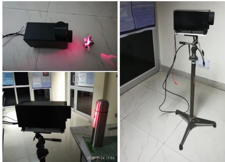
Developed portable digital holographic camera
