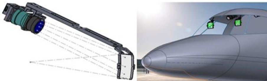
Layout of Head Up Display in Passenger Aircraft
