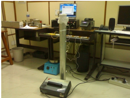
Experimental and schematic set up for distributed temperature monitoring of soil.
