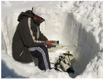
Field Trial of Snow Moisture Measurement System in progress
