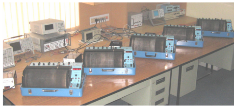
Analog Seismic Recorders under long term testing
