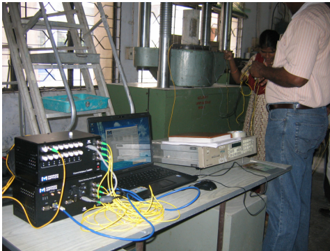
Setup for measuring compressive load using FBG sensors on a concrete specimen
