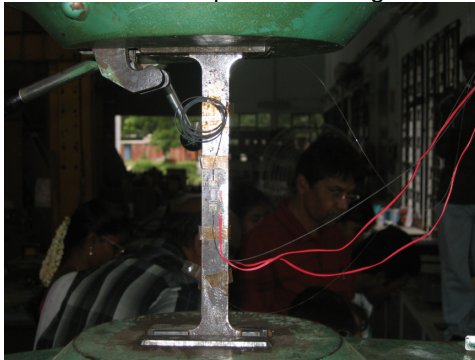
Tensile Strain Measurement on MS Specimen using both the CSIO-Developed FBG Sensor and Micron Optics FBG sensor with Electrical Strain gauge
