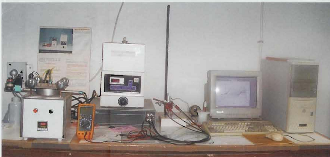
Computer Controlled Set-Up for Off-Flavour Measuring System
