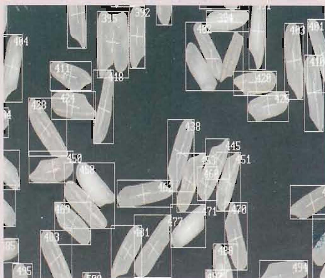
A part of typical image after blob analysis showing each kernel labelled uniquely.
