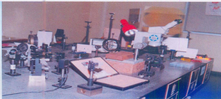
Experimental set up for fabrication of EFPI sensor
