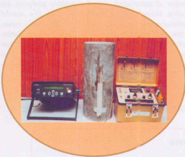
EFPI sensor and conventional strain gauge bonded to a concrete cubical specimen cast at PEC
