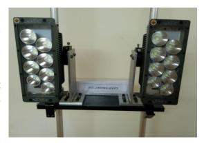
Undercarriage and the other on the Starboard (RH) side. Taxi &Landing Lights have three modes of operation i.e. OFF mode, Taxi Mode and Landing Mode. This Light operates on Aircraft nominal power supply i.e. 28V DC. CSIR-CSIO has developed the Taxi and Landing Lights along with its Indoor and Outdoor Test Rigs.
