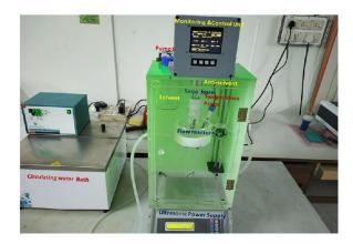
Working prototype of semi automatic and flow temperature control ultrasonic spray system consists of (i) power Ultrasonic supply sonohorn probe (ii) Double wall glass reactor with inlet and outlet (iii) Probe Temperature (iv)Microcontroller based monitoring and control module (v) Peristaltic Pump 1 & 2 (vi) Reagent Bottle 1 (solvent) & 2 (anti-solvent) (vii) mechanical assembly for support and adjust the position of reactor (viii) Circulating water bath
