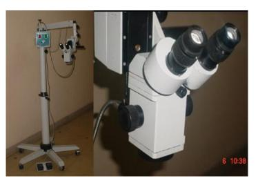
and four step magnifications is achieved through use of two telescopes of desired power in direct and reverse direction. The equipment has an excellent resolution with contrast facility, uniform illumination with large working area to the eye surgeons. In addition to this, the system also gives a true stereoscopic observation, modular construction, adjustable inter papillary distance and camera attachment facility for visual display.
