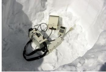
as sensor. Resonant frequency & 3dB bandwidth of sensor in snow are measured. These electrical parameters are used to determine the complex dielectric constant of snow. Furthermore, the density (0 - 0.6 g/ccm) & liquid water content of snow (0 - 15 % (Vol)) are calculated using empirical equations. All the computations are performed by microcontroller based electronic unit.
