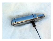
and molecules within the matter. As the temperature of the object increases, the molecular activity in the object increases causing the object to generate more energy. By using this concept, CSIR-CSIO has designed and developed an infrared technique-based snow surface temperature sensor which measures the snow surface temperature using non-contact remote sensing method. It can be easily interfaced with any automatic weather station.
