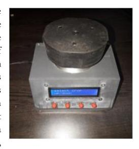
high speed microcontroller (MCU) chip for control and various processing applications. The sensing system is made up of impedance cell that converts moisture contents into corresponding impedance variations. Presence of a very small quantity of water causes considerable change in the impedance cell.
