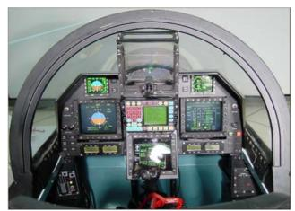
CSIO built Head UP Display Mk1 in LCA-AF Cockpit
