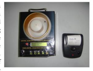
dielectric constant of the sensor cell. These moisture variations change capacitance which in turn is measured in terms of frequency variations. These variations are then further linearized and calibrated in terms of percentage moisture. The final result in terms of moisture percentage, temperature of sample, date and time of measurement is displayed on LCD for a given sample under measurement.
