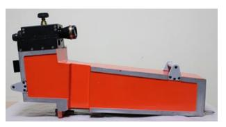
used to install and harmonize cockpit display and optronic systems at the desired position in the aircraft cockpit with reference to the aircraft axis (Fuselage Reference Line - FRL). It provides harmonization capability within tolerance of 1mR for harmonization distance of 60m. With this accurate harmonization, the target positioning for these Optronic Equipment would be within 9 feet for a distance of 20 kms.
