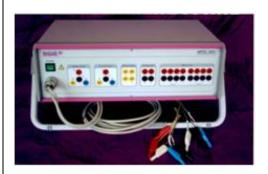
To generate simulated AC Power to test the 3 phase loads(3kVA each phase and also single phase load upto 9kVA
