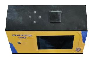
concentration of nitrate in the water sample. A minimal quantity of nitrate in water causes a considerable change in the detector's output. These variations are then further linearized and calibrated in terms of concentration (ppm). The final result in terms of nitrate concentration is displayed on the touch screen for a given sample under measurement.
